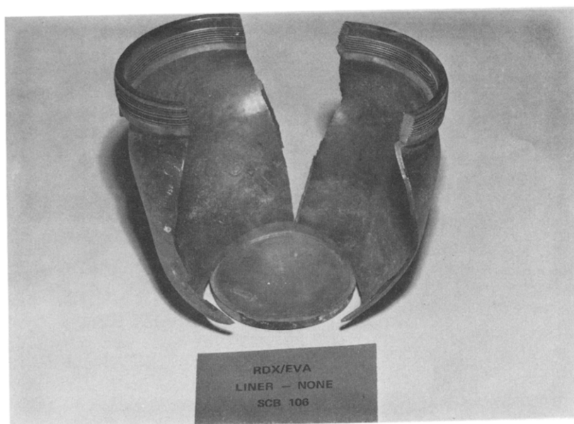
FIGURE 8b. MOLDING POWDER SECTION RDX/EVA A-3 (C 6 H 6 ) DEFLAGRATION.
