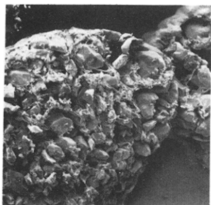
FIGURE 10a. MOLDING POWDER SECTION RDX/EVA 95/5 ( C_6H_6 ). NOTE: ORIGINALS 9 X 10 CM.
